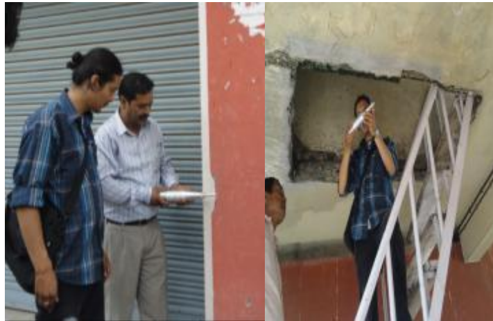
Figure 5-3 Carrying out Schmidt hammer test
