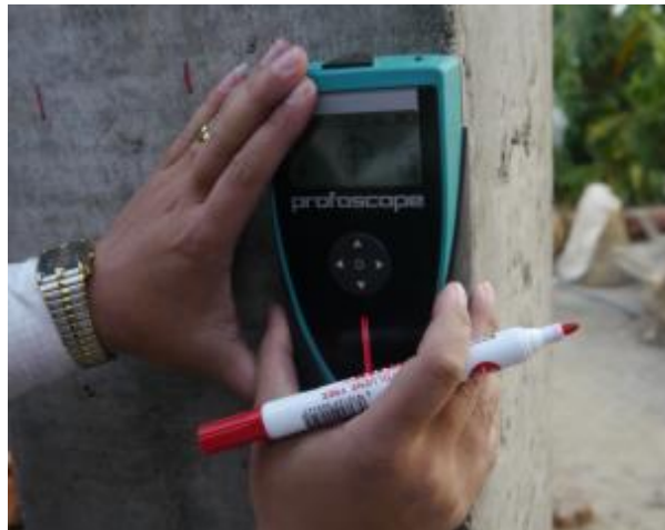
Figure 5-5 Cover meter and rebar detector test
