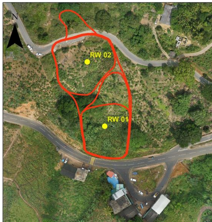
Figure 4-4 Landslide foot print at Galabada
