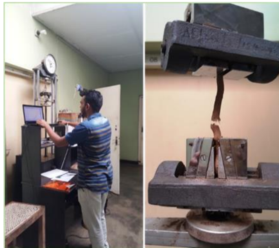
Figure 6-2 Root tensile strength testing using Dynamometer
