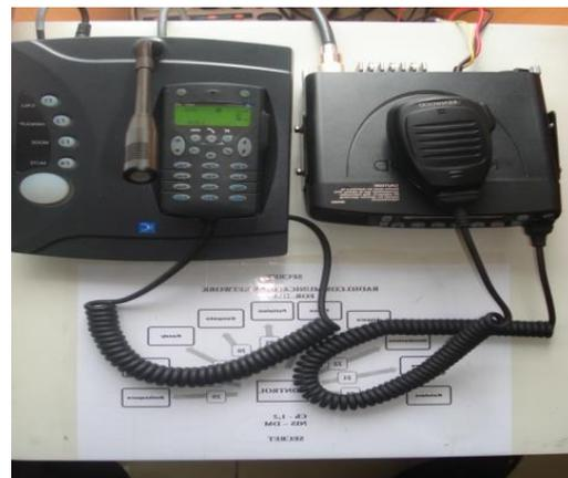
Figure 22: Radio Communication system in Vehicle
