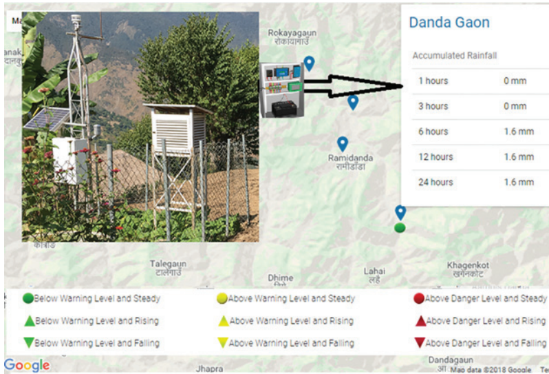
Figure 11. Existing real time data transmission system with online acquisition
